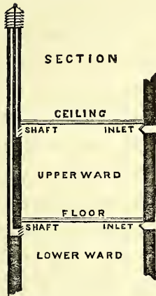
Section of Ward Ventilation.
